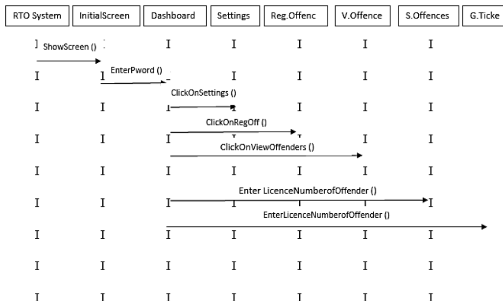
Figure 5. Sequence Diagram of Road Traffic Offence Information Management System
