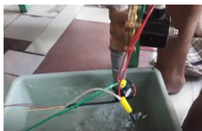
Gambar 24. Pengujian Water Flow Sensor
