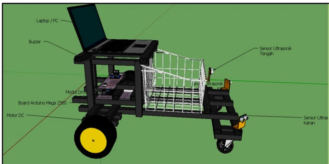
Figure 1. The design of the trolley robot
