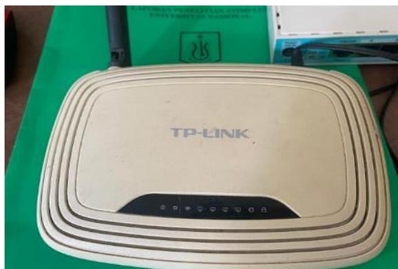
Gambar 6. Router TP-LINK TL-WR740N
